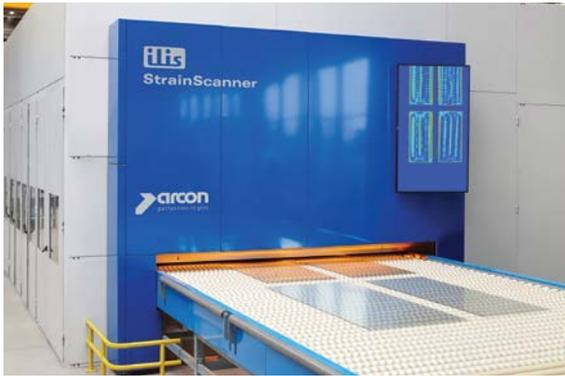
Figure 5: In co-operation with arcon, the first inline StrainScanner was installed in Feuchtwangen for the objective and continuous measurement of the quality of toughened safety glass (photo courtesy of arcon).
