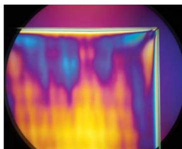
Figure 1: By using crossed polarising filters, brightening in areas with residual stresses are visible in the polariscope picture of a tempered glass pane (left image). When using white lighting (right image), interference effects result in a coloured picture.
