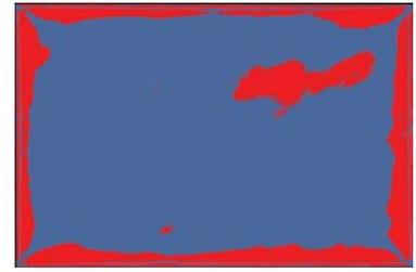
Figure 6: Based on the measured vectorial stress data of a glass pane (left image), the anisotropy simulation visualises unwanted anisotropic effects under the most unfavourable lighting conditions.
