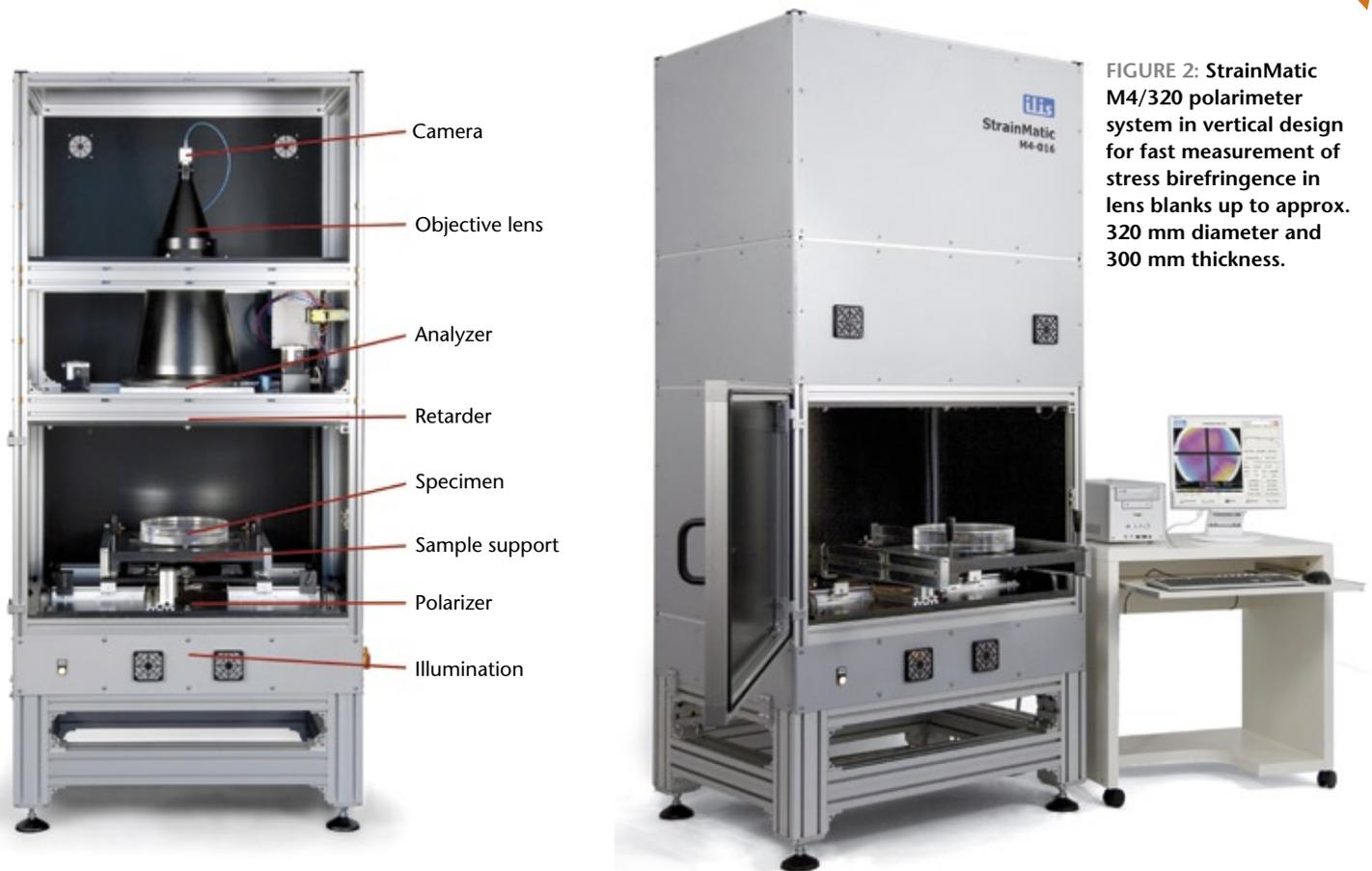
**FIGURE 2:** StrainMatic M4/320 polarimeter system in vertical design for fast measurement of stress birefringence in lens blanks up to approx. 320 mm diameter and 300 mm thickness.
