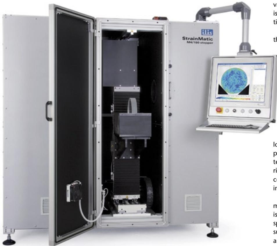
FIGURE 4: StrainMatic M4/160 polarimeter system in horizontal design with fully automatic stitching for specimen measurements up to 400 x 400 x 100 mm<sup>3</sup> and 100 kg weight.
