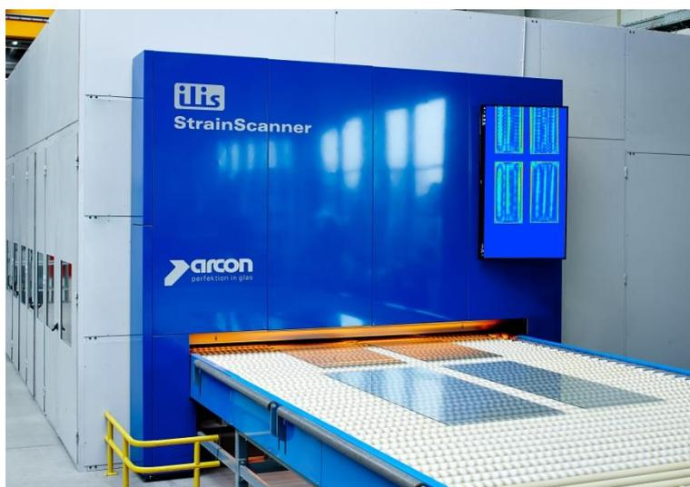
**Caption:** The StrainScanner performs a photoelastic measurement of the glass panes in real time and analyses them with regard to anisotropy. (Source: arcon)
