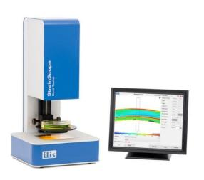
**StrainScope® Cord Tester**Cord stresses in container glass
