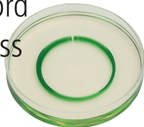
▲ Fig 1. Ring section of a beverage bottle in a petri dish filled with immersion liquid.
