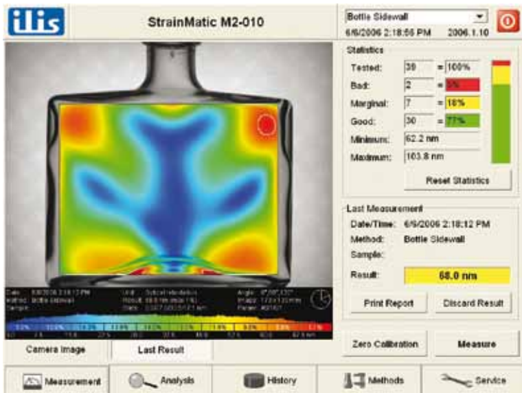
FIGURE 4: THE STRAINMATIC'S OPERATOR INTERFACE WITH MEASURING RESULT
